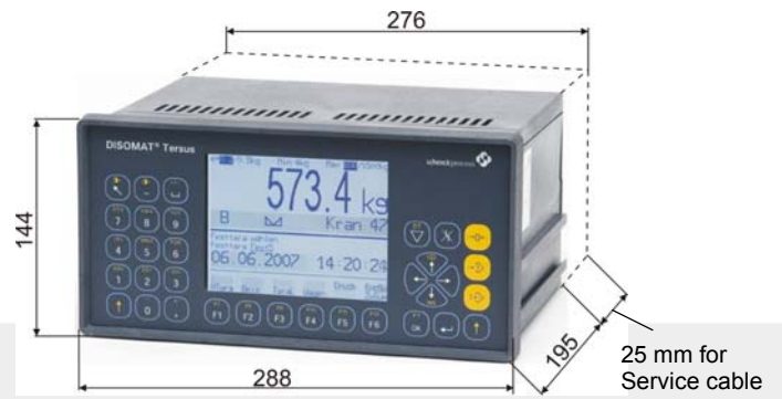
Panel-mount VEG 20450 terminal Protection class: front IP54, otherwise IP 20 plastic 138.5 x 282 mm panel cut-out, weight: 3.5 kg
