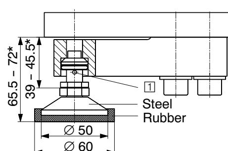
① Foot fixed in the load cell with the enclosed spring shackle
