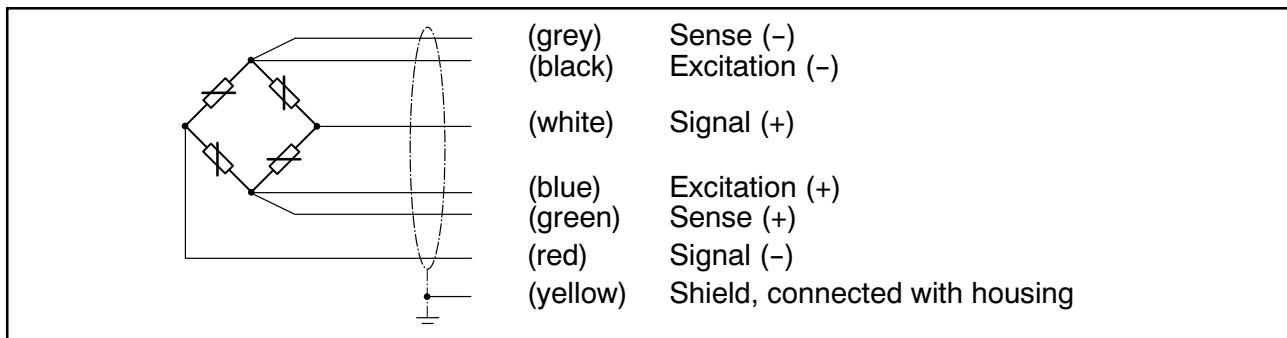
When connecting 6-wire load cells to amplifiers in 4-wire technique you must connect the wires **blue to green** and **black to grey** are to be connected up. The following deviations occur on **unshortened** cables (3 m):
