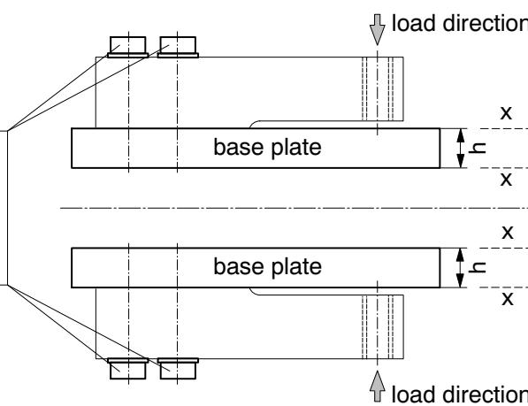
The base plate should be made from stainless steel, with a Rockwell hardness of 42. The surfaces "X" must be even and in parallel (0.25 mm).
