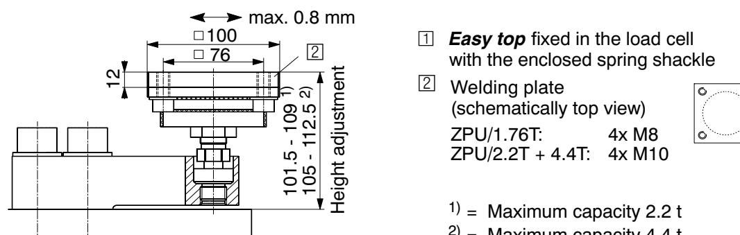
**HLC/ZPU/...T** – Base plate / Mounting kit (galvanized material)
