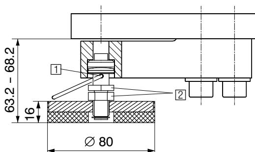
① Foot fixed in the load cell with the enclosed spring shackle
